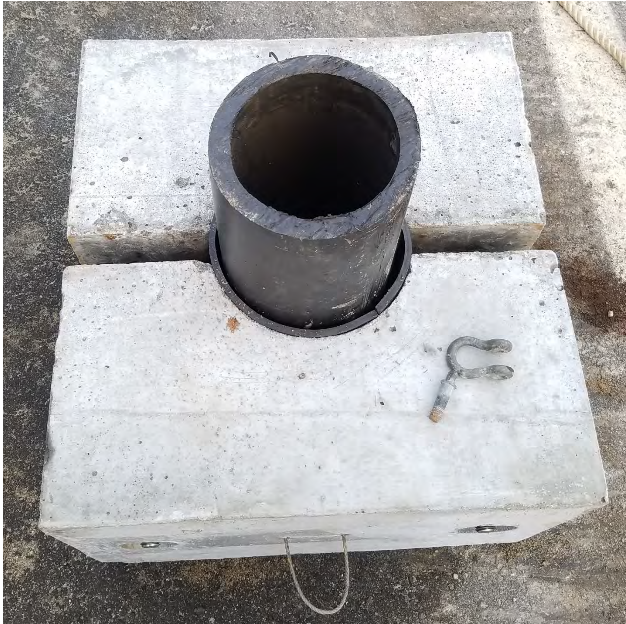
11: 300-lb. weight installed on test section of pipe
